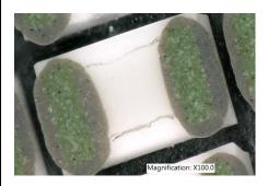
Arter cleaning, this precise jig is evaluated under optical alds for remaining residues under components.
